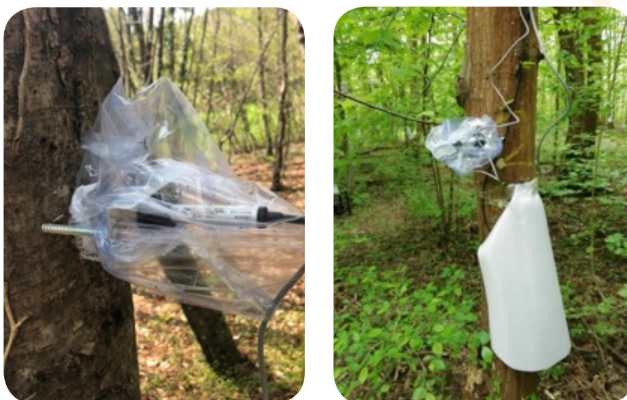
Figure 2. In the first picture, dendrometer on hop hornbeam in Caltrano. In the second one, dendrometer on Carpinus betulus in Carlino, covered with a plastic bag to prevent moisture damage. Credits: Enrico Vidale and Alessia Sartori.
