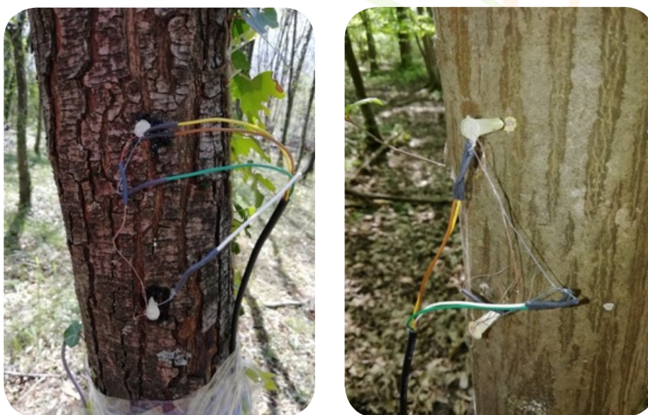
Figure 1. Granier sensors in the sites of Caltrano (on Ostrya carpinifolia ) and Carlino (on Carpinus betulus ). Credits: Alessia Sartori.
