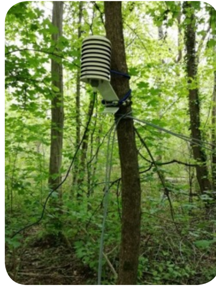
Figure 3. Hygrometer in the sites of Caltrano (left) and Carlino (right). Credits: Alessia Sartori.
